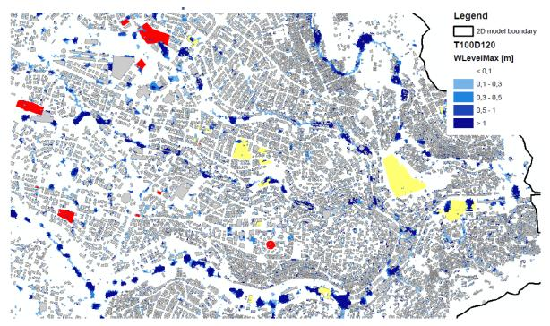
**Figure 10.** First risk map for Downtown Amman. Results of the hydro-dynamical 2D simulation with the model HE2D/FOG2D and building usages with a high (yellow) and a very high (red) damage potential are shown.
