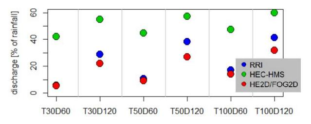
**Figure 12.** Total runoff volumes modelled with RRI, HEC-HMS and HE2D/FOG2D for design storm events with different return periods (T) and durations (D) for a subbasin of the Wadi Musa catchment  $(A_E = 18.5 \text{ km}^2)$ .
