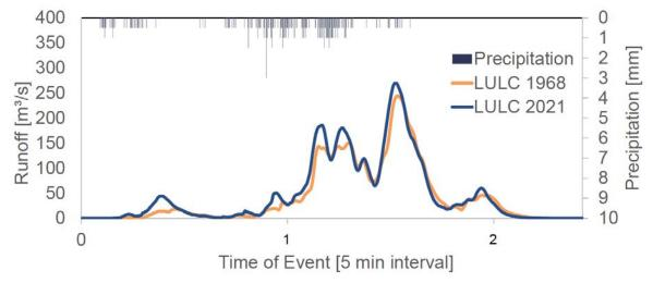
**Figure 11.** Modelled runoff of the hydrological model HEC-HMS. The two days rainfall event from February 2019 (5-minute resolution of rainfall series) was modelled with the LULC 1968 (yellow) and the LULC 2021 (blue).
