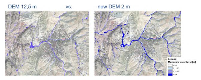
*Figure 7.* Results of the hydraulic model HE2D/FOG2D for the area of Wadi Musa / Petra. On the left based on the DEM with a resolution of 12.5 m and on the right based on a high resolution DEM of 2 m.
